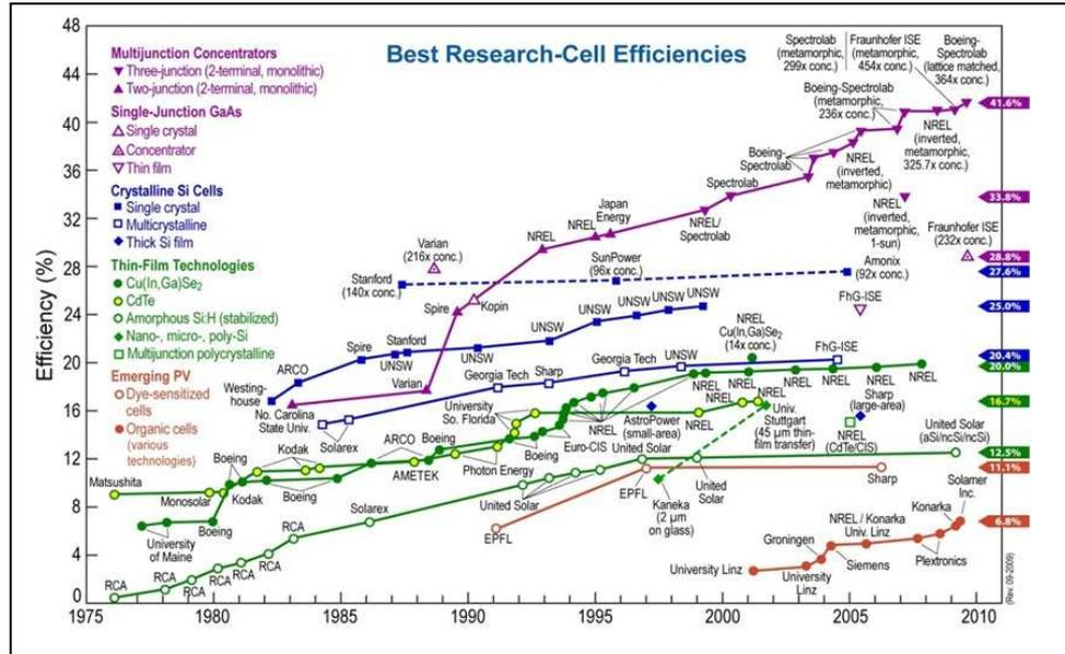
Figure 2: Performances of different solar cells
